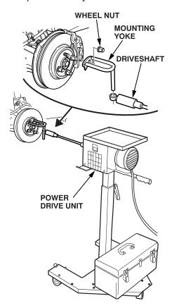
3. Attach the driveshaft on the drive motor assembly to the mounting yoke, making sure the center line of the driveshaft is level with the spindle nut on the wheel hub.
