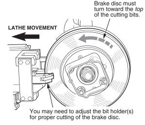
Do not set the cutting depth on the brake lathe to more than **0.2 mm (0.008 in.)**. This is *two* divisions on the cutting knob. Make sure you start your cut at least **3 mm (0.12 in.)** beyond the worn area on the brake disc.
