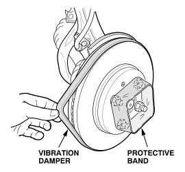
If you are not using the power drive system, use a fabric tie-down strap to secure the brake disc that is
