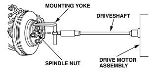
4. Set the lower toggle switch on the drive motor assembly to **FWD** (counterclockwise rotation) or **REV** (clockwise rotation).
