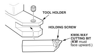
Before you use the brake lathe, inspect the tips of the cutting bits with a magnifying glass to make sure the tips are not worn out. Each bit has three tips. If a tip is worn, rotate the bit, and use a new tip. A worn tip produces a poor finish and may cause chattering.
