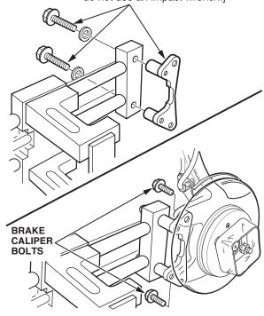
[Torque to 54 N·m (40 lb-ft); do not use an impact wrench.]
